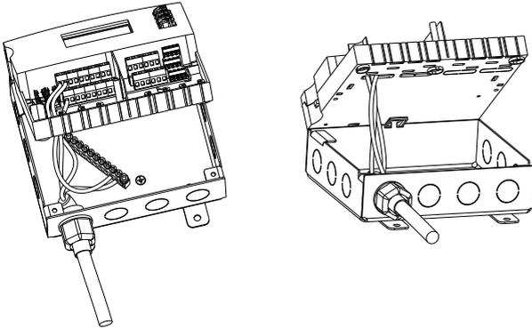
Unscrew the controller from the metal tray before installation. Use a suitable tool to break out the pre-punched holes which are required for the installation.
